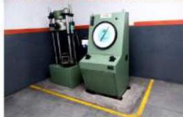
Tensile and Elongation Testing Capacity: 40 Tonnes
